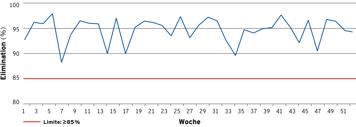
TOC/DOC-Elimination ARA Chemie 2023
